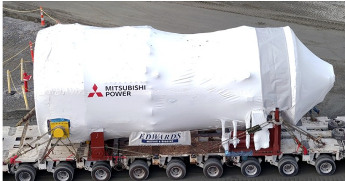
A new natural gas turbine is delivered to Plant Yates in Newnan. The turbine weighs nearly 350 tons, is 50 feet long and 18 feet wide
